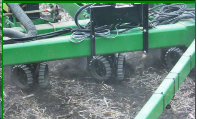
Below: See the Yetter residue managers cleaning off the strip ahead of the planter row unit.
