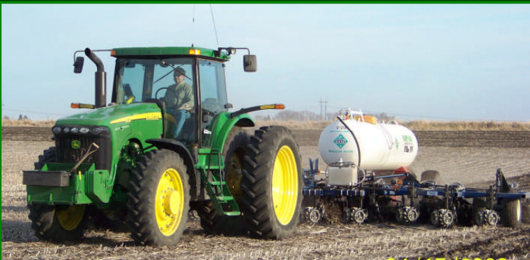
Gary Applying NH 3 to the Haire South Farm. We use our Strip Tillage machine to also Variable rate our NH 3 .
