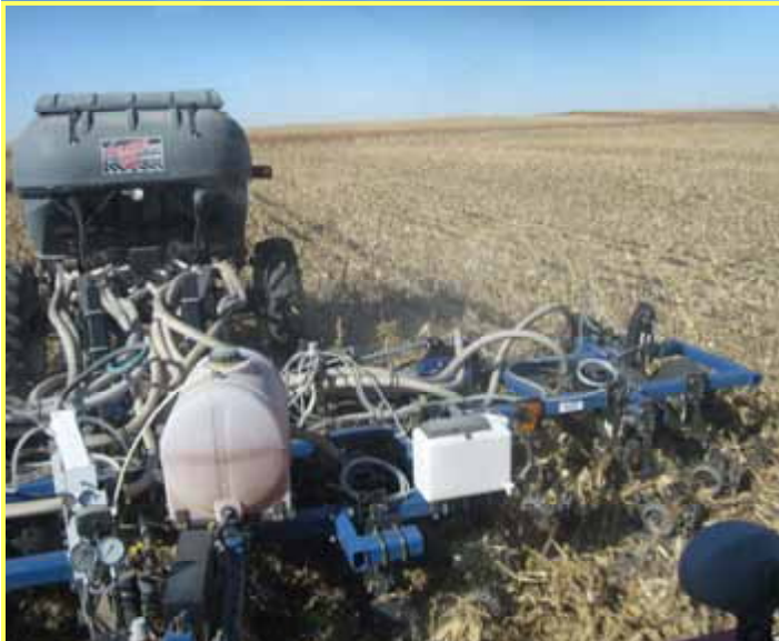
Above: Our Blu-Jet/Montag strip till machine applying Nitrogen, Potassium, Phosphorus, and N-Serve in the fall.
