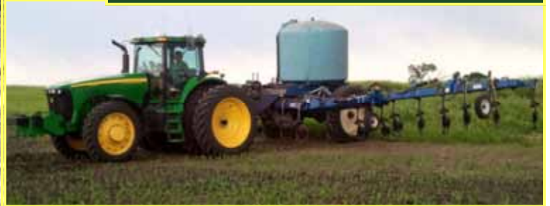
Right: On our Blue-Jet Sidedresser we use the Capstan variable rate injection system. From 5 gpa to 70 gpa with no changing of the orifices.
