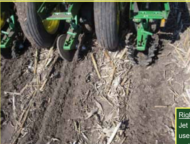
Above : Comparing closing wheels on the planter this spring. Dawn Curvetine on left and Yetter's on right.
