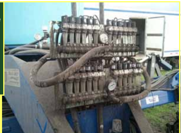
Right: On our Blue-Jet Sidedresser we use the Capstan variable rate injection system. From 5 gpa to 70 gpa with no changing of the orifices.
