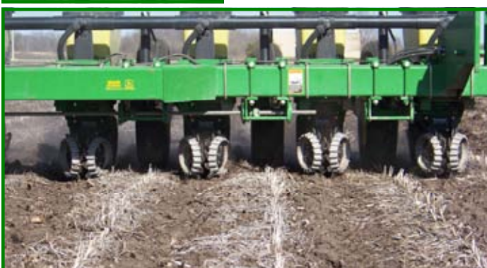
With the help of RTK Auto Steer and the sub-inch accuracy, see how the planter follows the strips made last fall.
