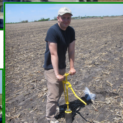
An ISU grad student pulls soil cores on the Smeltzer #4 farm to look at soil drainage, compaction and profile.
