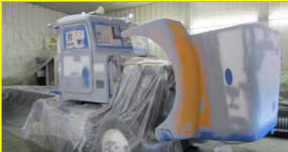
Above: Peterbilt tender truck: sanded down, primer applied, now waiting for the shiny red paint.
