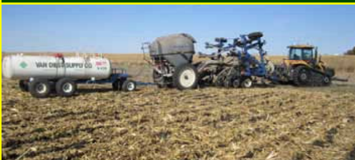
Above: A view of our strip till rig folded up and ready to go down the road. 100% of our tillage and fertilizer is done in the fall!
