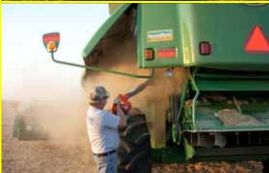
Above: Gary blowing the dust out of the combine to prevent a fire from starting. A dirty job.
